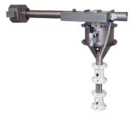
Another popular metal detector—particularly in bulk food applications such as sugar or flour—is the Bunting pTRON™ series of metal detectors. Bunting pTRON metal detectors can be placed in horizontal or vertical piping moving powdered material. Now available for use in pipe as large as 8 inches in diameter, pTRON detectors provide the same assurance as Bunting meTRON detectors, but for bulk materials being transferred from place to place.
